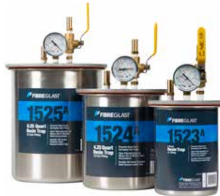
Each Resin trap come complete with glycerin-filled vacuum gauge, fittings for use with 1/2" vacuum tubing, brass ball valve and instruction manual.
